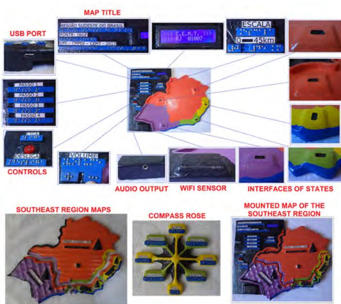
Figure 3 - Tactile map CEMT and its components.
