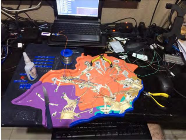
Figure 1 - Installation of Sensors on the CEMT Touch Map.
